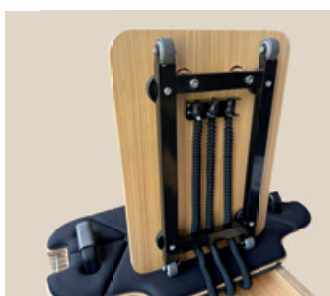
When connecting the three ropes, they must be inserted into the holes of the metal plate.
